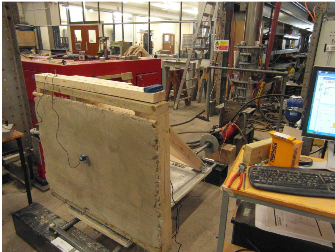
Figure 6: Set up for out-of-plane testing of wall panels on a uni-directional shake-table at Cambridge University (Kaminski, 2014).
