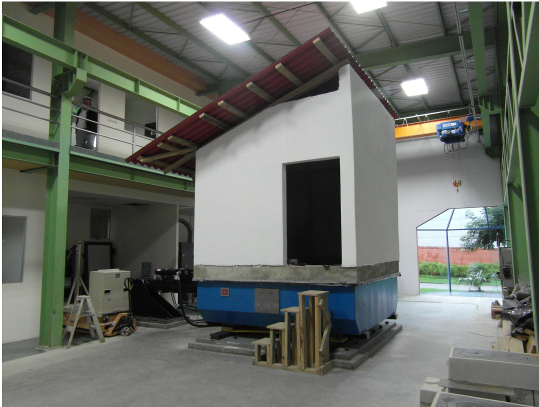
Figure 7: Completed full-scale room of a house at the Universidad Mariano Gálvez in Guatemala City, ready for bi-directional shake-table testing (Kaminski, 2014).
